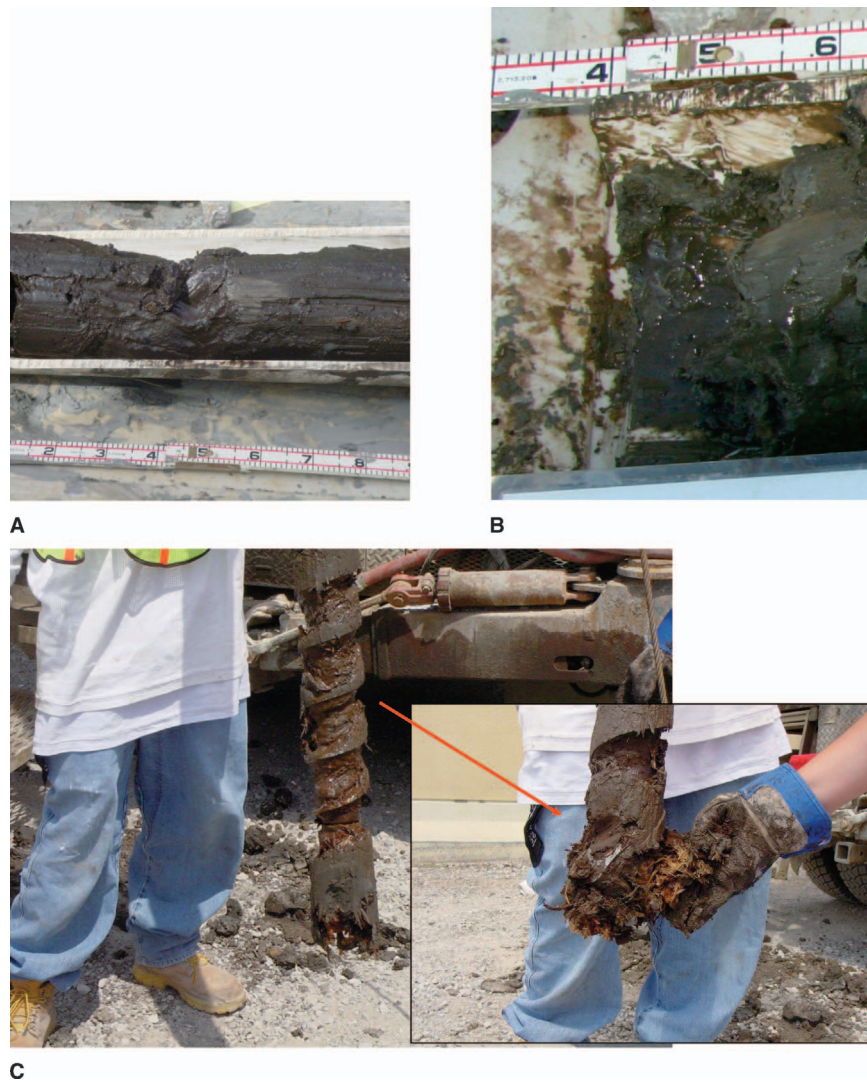
Fig. 14. (Color) (a) Sheared sample of the sensitive organic silty clay layer from within the slide area; (b) unshereed sample of the same material from near to the slide area, but not within it; and (c) shiny dark brown to black sensitive organic clay on auger stem and (inset) closeup view of layers of leaves and twigs—17th Street Canal breach site
